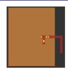
The Monopole antenna is fabricated using a conventional PCB process, featuring a dielectric constant of 4.6 and a loss tangent of 0.01. It has a profile height of 1.6 mm, a metal thickness of 0.035 mm, and operates at 2.40 GHz. Impedance matching for the antenna is achieved through the utilization of a lumped circuit elements.
